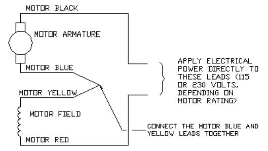
MOTOR CONNECTIONS FOR "IN" DIRECTION
