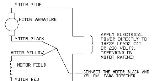
MOTOR CONNECTIONS FOR "OUT" DIRECTION
