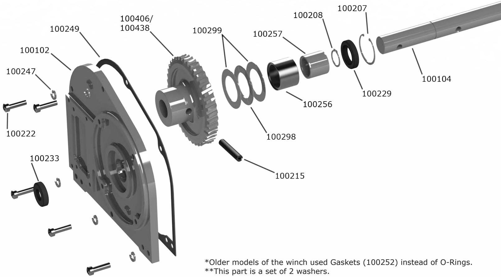
\*Older models of the winch used Gaskets (100252) instead of O-Rings.
